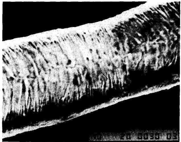
Fig. 8. Permalloy fibre treated to a grain boundary etch showing the growth of crystallites away from the line of contact with the wheel.
