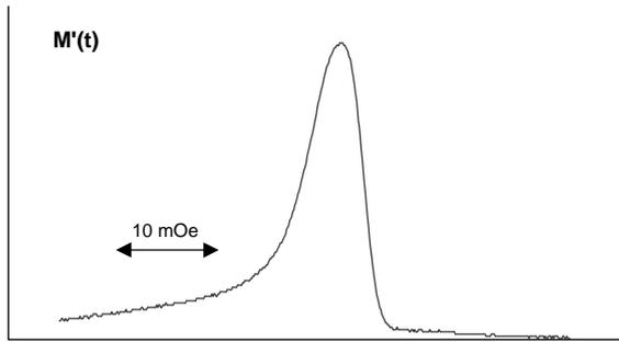
Fig. 5. The measured  $M'(t)$ , taken directly from an oscilloscope output, through its maximum in a sinusoidal driving field of amplitude 3 Oe and frequency 500 Hz. The scale for  $M'(t)$  is arbitrary.
