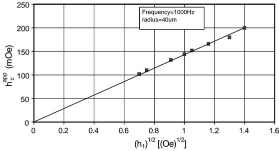
Fig. 2. The apparent coercivity as a function of the amplitude of the sinusoidally varying driving field. The line is a least-squares fit through the points.
