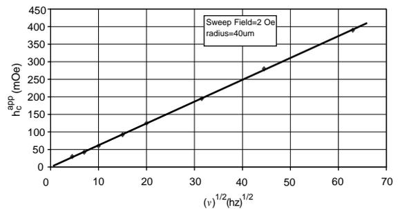
Fig. 1. The measured coercivity against square root of the frequency. 1 Oe is approximately  $80 \text{ A m}^{-1}$ . The square-root dependence continues at least up to 20 kHz. The line is a least-squares fit through the points.
