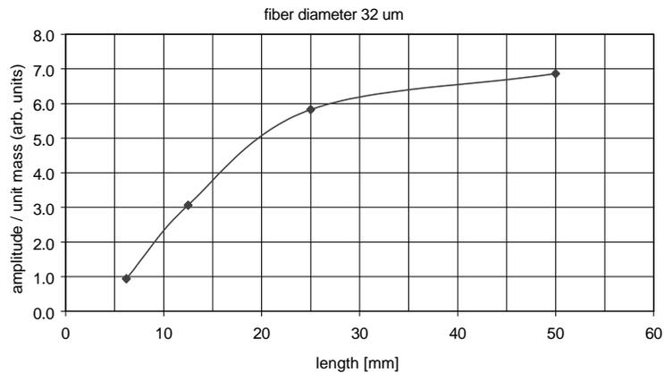
Fig. 4. Effect of length on the amplitude of  $M'(t)$ . The amplitude of the driving field was 2.5Oe and its frequency 5 kHz.
