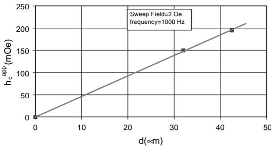
Fig. 3. The apparent coercivity as a function of fiber diameter. The line is a least-squares fit through the points.
