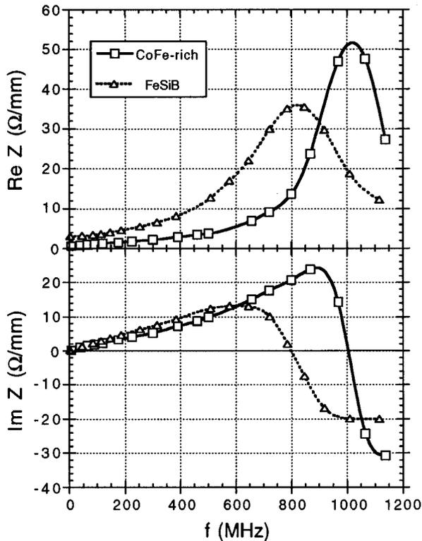
FIG. 3. Real and imaginary parts of the impedance of CoFe-rich and FeSiB fibers as functions of the frequency. The applied field was 120 Oe. Re Z peaks and Im Z crosses zero at the same frequency for each fiber. Cubic spline fitting was used again.
