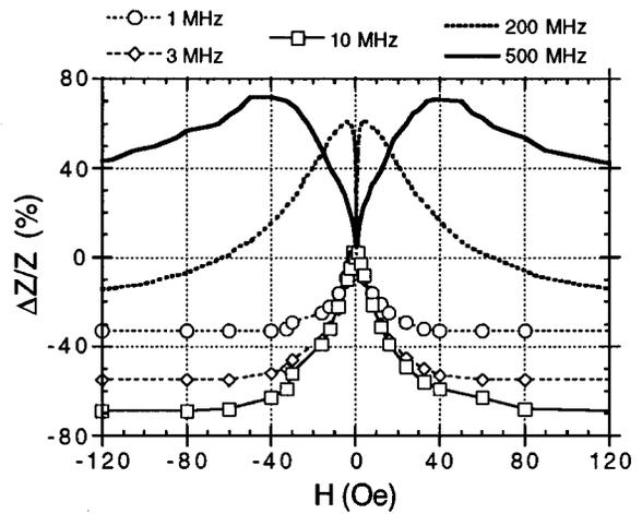
FIG. 4. GMI responses of a NiCo-rich fiber for frequencies ranging from 1 MHz to 500 MHz.
