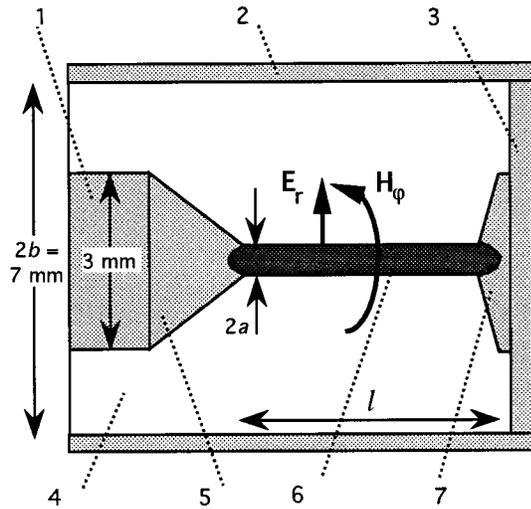
FIG. 1. Longitudinal cross-section of the coaxial line used to measure the GMI effect from 1 MHz to 1.2 GHz: (1) inner conductor, (2) outer conductor, (3) short-circuit piston, (4) air, (5) matching transition (conductor), (6) magnetic fiber, (7) conductor. Propagation modes and spatial distribution of the field components are also shown.
