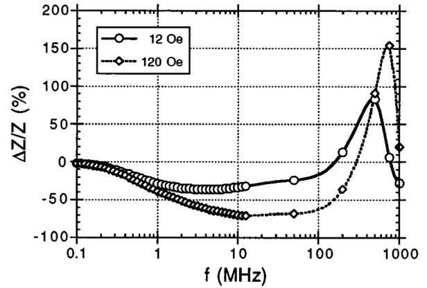
FIG. 2. GMI spectra of a NiCo-rich fiber for two dc axial magnetic fields. Data from 1 kHz to 13 MHz have been obtained with an impedancemeter. Data from 5 MHz to 1.2 GHz have been obtained with an impedance analyzer, using the setup in Fig. 1. In the latter case, the spectra have been plotted using a cubic spline curve fit.
