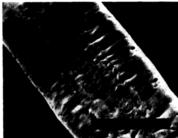
Fig. 1. SEM micrograph of a NiFe fiber showing the contact line.
